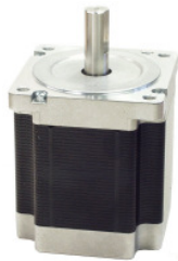
Motor: sm296ht-KF7.0A-008 Drive:smd276 Umotor: 24V, 48V, 72V Inom: 7.0A Imax:8A 1000 Steps/Rev
