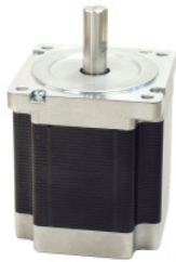
Motor: sm296ht-KF7.0A-008 Drive:smd298 Umotor: 130V Inom: 7.0A Imax:8A 1000 Steps/Rev
